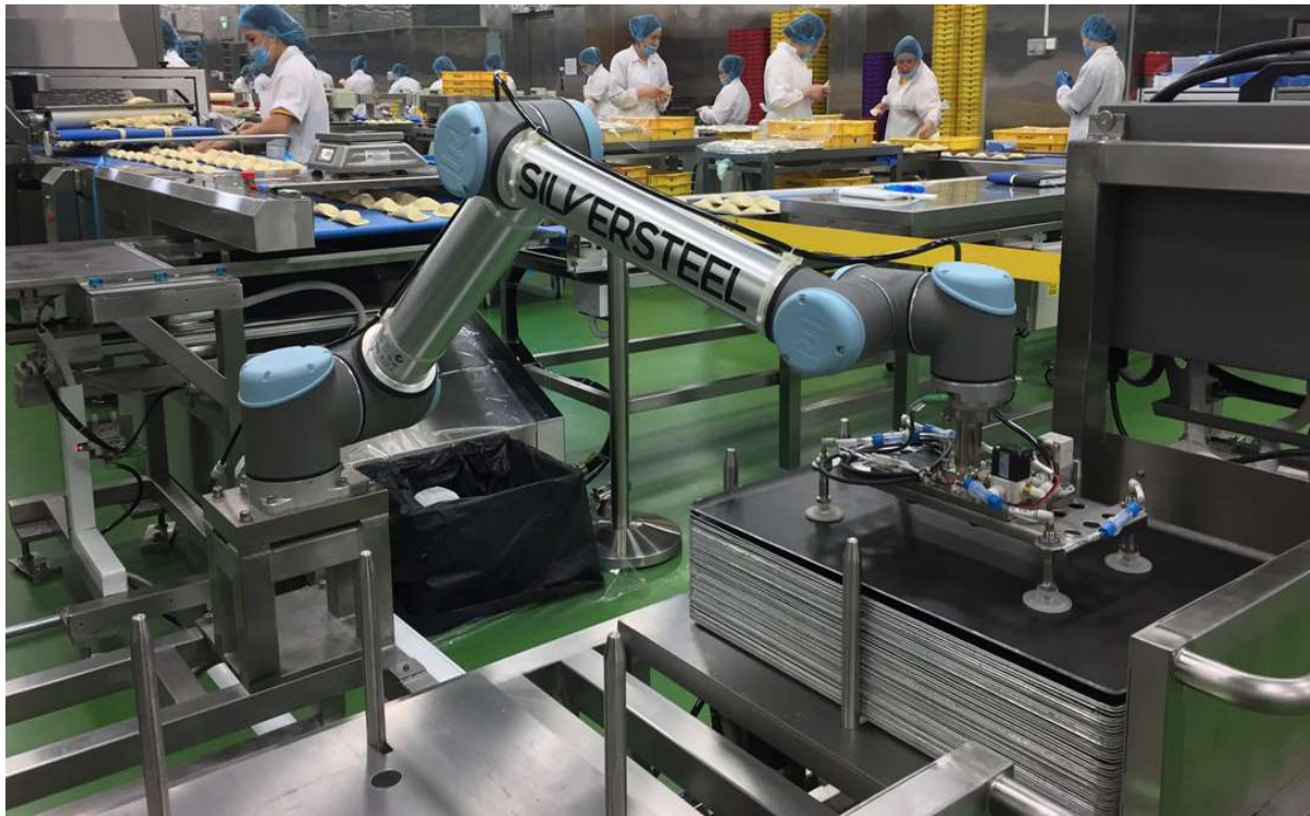
Pastry Production Robotic Tray Transfer System
